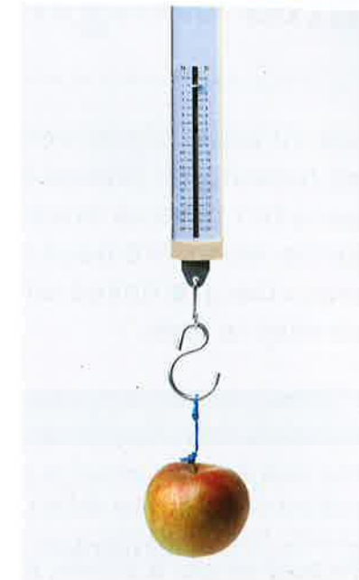
FIGURE 1.1.7c: All masses close to the Earth's surface are pulled by the gravitational field strength of 10 N/kg.
