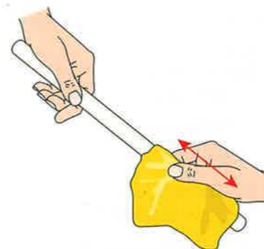
FIGURE 1.2.7b: Rubbing transfers electrons, either from the rod to the cloth or from the cloth to the rod.
