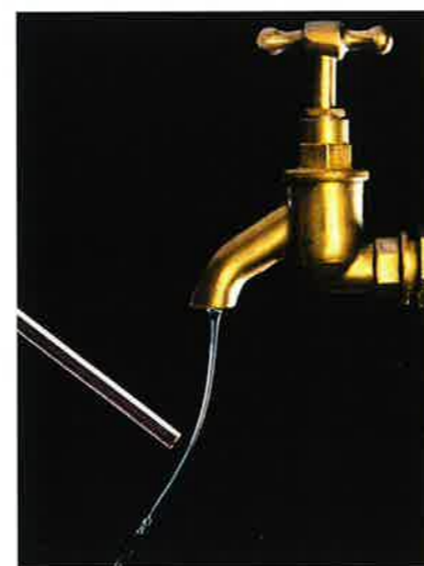
FIGURE 1.2.8a: The water is attracted towards a charged rod.
