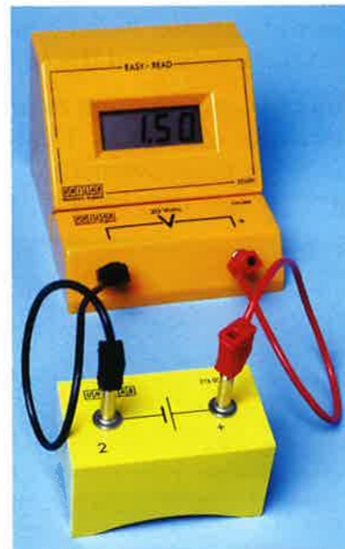
FIGURE 1.2.2a: A voltmeter is a tool to measure voltage, but what do we mean by voltage?
