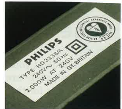
FIGURE 1.3.2d: The power rating of the electric fan heater is shown on the label. It is 2000 W.
