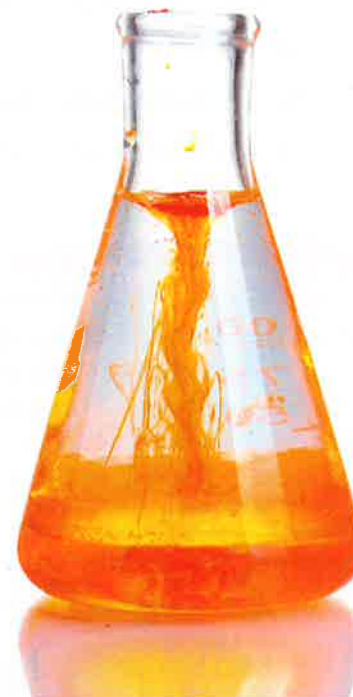
FIGURE 1.5.4a: If a drop of coloured ink is added to water, after several hours the colour will have spread through the water so that it is of equal concentration throughout.
