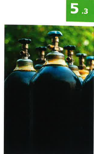
FIGURE 1.5.3b: The cylinders contain gas which has been liquefied. When released, the change in pressure causes the liquid particles to become gas particles again.
