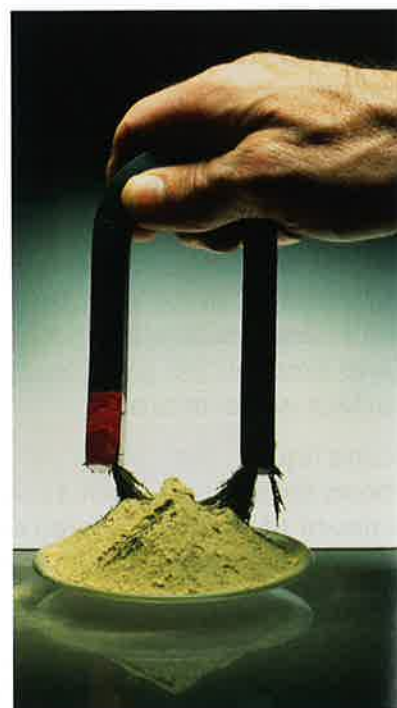
FIGURE 1.5.6b: The physical property of magnetism can be used to separate magnetic from non-magnetic materials.
