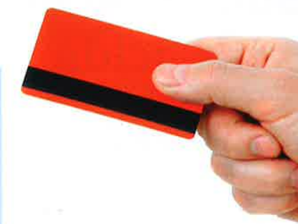
FIGURE 1.6.1c: Credit cards contain a magnetic strip which encodes information about its owner.
