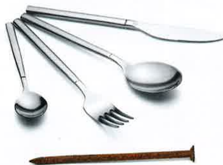
FIGURE 1.6.1b: Stainless steel is an alloy of iron that doesn't rust.
