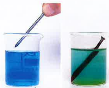
FIGURE 1.6.3b: Iron and copper sulfate solution – before and after the displacement reaction. Over time, the blue copper sulfate solution becomes paler, and the iron nail becomes covered with a brown coating of copper.
