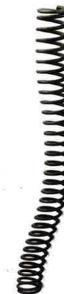
FIGURE 2.1.4c: This spring has been stretched beyond its elastic limit.
