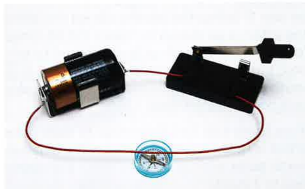
FIGURE 2.2.3a: When the switch completes the circuit, the compass needle moves – the current in the wire is acting like a magnet.
