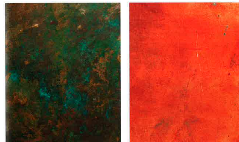
FIGURE 2.4.1d: Before (left) and after (right), the ultrasonic cleaning of a piece of old copper plating.
