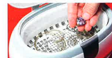
FIGURE 2.4.1c: Jewellery can be cleaned by ultrasound. The object is put in a dish of liquid and the ultrasound makes it vibrate for several minutes.
