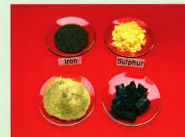
FIGURE 2.5.10b: Iron (top left), sulfur (top right), iron and sulfur mix (lower left) and iron sulfide (lower right).
