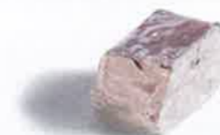
FIGURE 2.5.2b: Sodium is a soft reactive metal.
