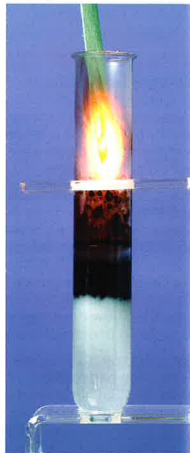
FIGURE 2.6.4a: Decomposition of hydrogen peroxide can be catalysed by manganese dioxide (black powder) to form water and oxygen. The oxygen allows a flame to burn on the wooden splint.
