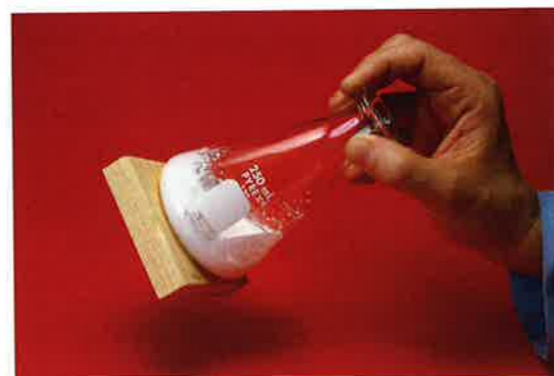
FIGURE 2.6.2b: When an ammonium salt is dissolved in water, the temperature drop is enough for ice to form on the outside of the flask.
