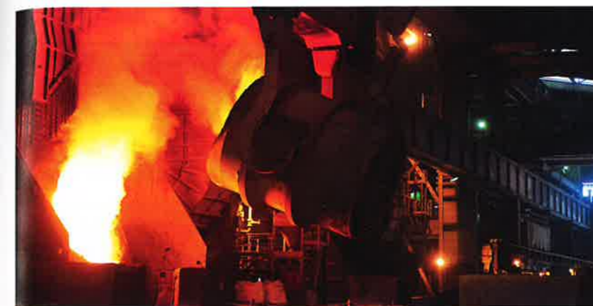
FIGURE 2.7.7c: Making iron involves heating the ore strongly with coke. Other ingredients, such as limestone, are added to remove impurities from the iron. Air is blasted in and the temperatures are well over 1000°C.
