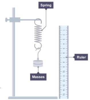
The **<u>extension</u>** of a material or a spring is its increase in length when pulled. Hooke's Law says that the extension of an elastic object is directly proportional to the force applied to it. In other words:
