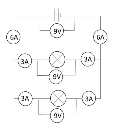
In a parallel circuit the potential difference is the same in all parts of the circuit regardless of how many loops there are. However, the current splits up between each loop. In the diagram below you can see how the total current flowing into a junction equals the total current flowing out from a junction.
