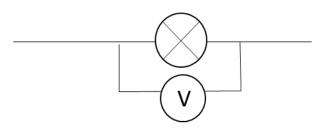
A <u>Voltmeter</u> measures the <u>potential difference</u> between two points in a circuit. It compares the energy that each unit of charge carries between two points in a circuit. In the same way that if you are comparing the height of two people you need to stand back from them, a voltmeter has to stand back from the circuit to make the comparison. It therefore must be connected in parallel with components in a circuit.
