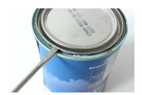
The pivot is the rim of the paint tin. The screwdriver rests on the pivot. There is a small length of screwdriver from the pivot to the paint tin lid. There is a large length of screwdriver from the pivot to your hand.
