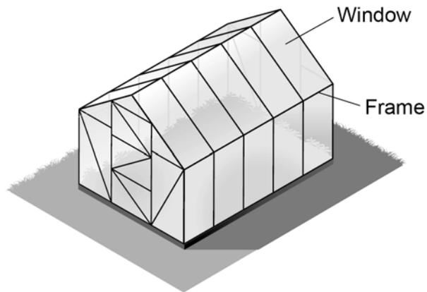
A greenhouse frame can be made from wood or aluminium.
