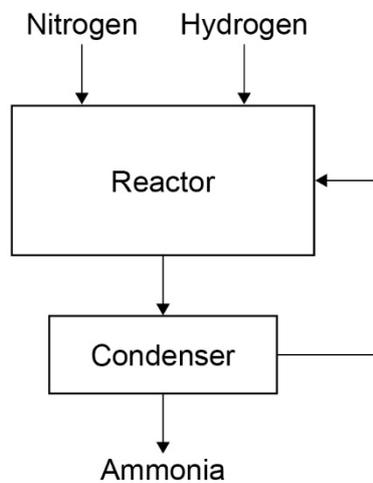
A mixture of ammonia, hydrogen and nitrogen gases leave the reactor.
