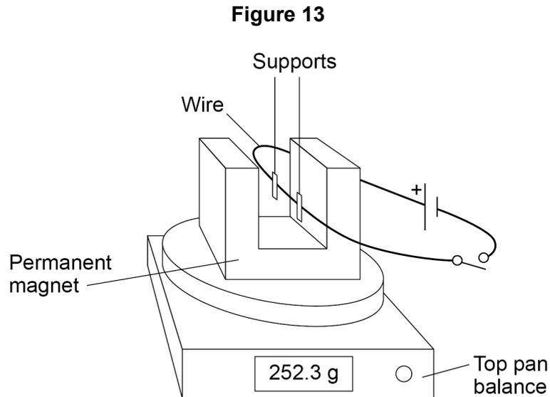
The top pan balance was used to determine the force on the wire.
