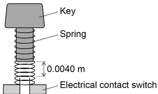
The key must be pressed with a minimum force of 0.80 N before the key touches the switch.
